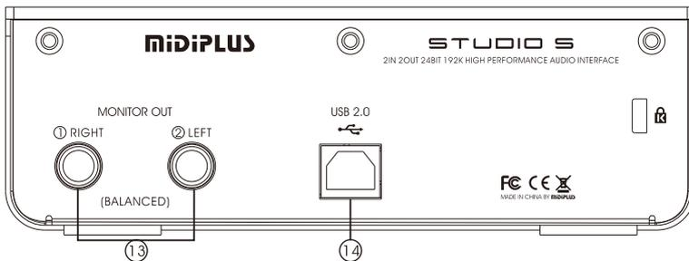
13. Monitor output interface: 6.35mm balance output interface
